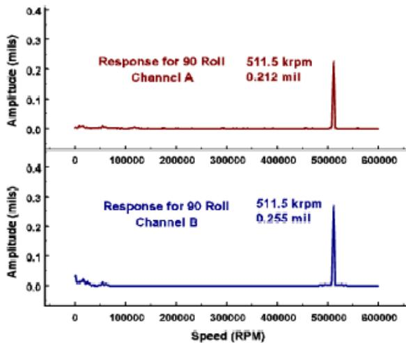
Fig. 10. Spectrum for 90° roll about spin axis.
