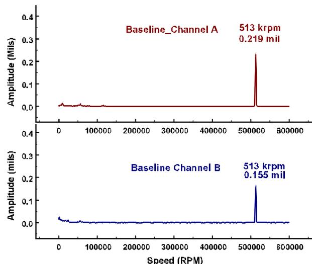
Fig. 9. Rotor vibration at 513,000 rpm for horizontal orientation.
