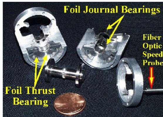
Fig. 1. Mesoscopic turbojet simulator rotor, split housing and MiTi<sup>®</sup> split air foil bearings.
