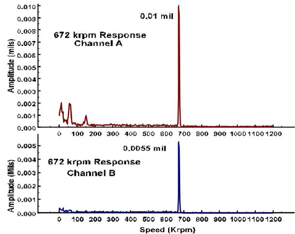
Fig 8. Spectrum for rotor at 672,000 rpm
