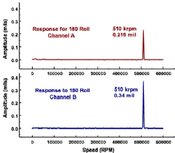
Fig. 11. Spectrum for 180° roll about spin axis
